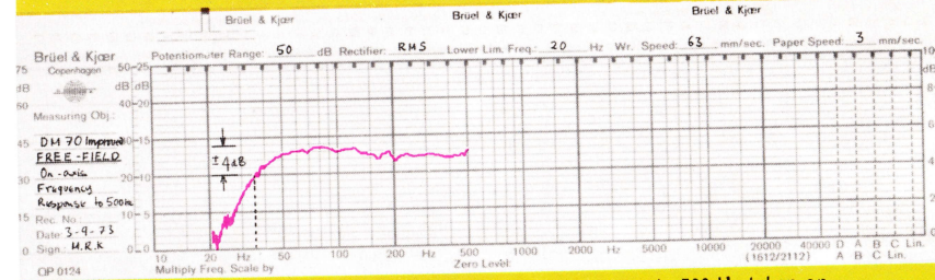
Free-field Frequency Response. Frequency response up to 500 Hz taken on 5 metre tower in open. Comparison with above plot shows limitation of Anechoic Chamber at very low frequencies only
