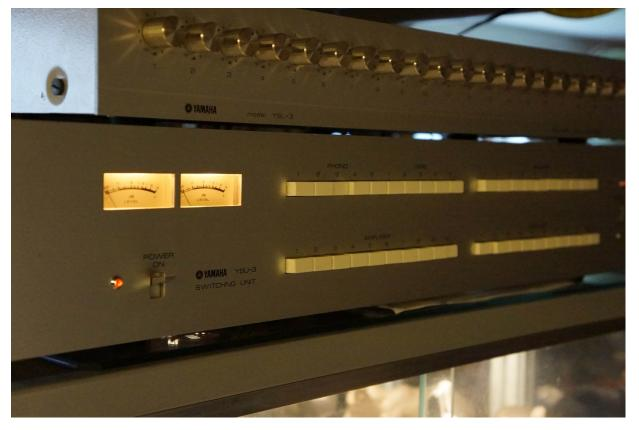
What is a switching unit? - Simply put, it allows you to connect every piece of stereo gear you've ever collected, all at once, and switch freely between any combination of components and any set of stereo speakers, up to 20! Internal Relay switches are used for everything so there is zero signal path loss and the power is unlimited.
