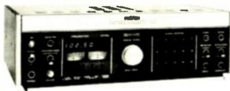
channels through pushbutton operation; five-digit LED front-panel display of station frequencies; variable muting and separation; Dolby-B card option available; logarithmic signal-strength and center-tuning meters; multipath scope output; 50-dB quieting sensitivity 2.5  $\mu$ V; capture ratio 0.9 dB; spurious, image, and i-f rejection 106 dB or better; mid-band separation 42 dB; AM suppression 75 dB; THD less than 0.15% (stereo and mono); S/N 75 dB; 6" H x 17 3/4" W x 13 3/4" D ..... \$1649
