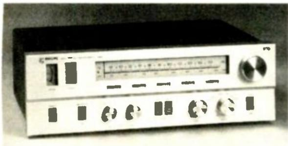
level controls; FM muting; LED touch switches. FM section: sensitivity 3  $\mu$ V stereo; 50-dB quieting sensitivity 2.2  $\mu$ V mono, 30  $\mu$ V stereo; capture ratio 1 dB; AM response -50 dB; i-f response -110 dB; image response -110 dB; stereo separation 50 dB (1 kHz); hum and noise -72 dB. AM section: sensitivity 150  $\mu$ V/m (rod antenna); image response -68 dB; i-f response -52 dB; hum and noise -60 dB. 5 1/2" H x 18" W x 13 1/2" D ..... \$530
