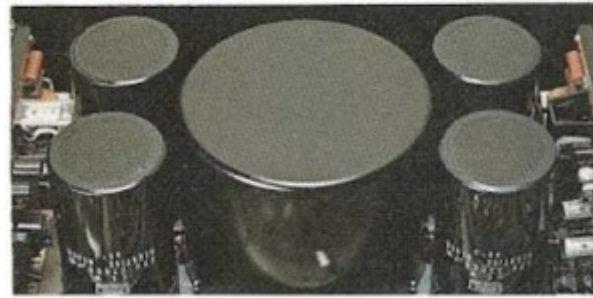
HUGE POWER SUPPLY SECTION WITH TOROIDAL-CORE POWER TRANSFORMER AND LARGE ELECTROLYTIC CAPACITORS
