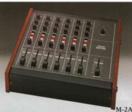
M-2A 6-In/4-Out Mixing Console
