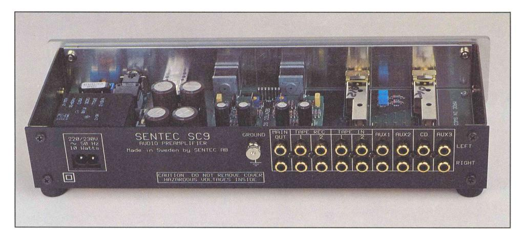
The SC9 is an all discrete design using high quality long-life components in a carefully wellthought circuit layout. As we do recommend short speaker cords with the power amplifiers close to the speakers, the SC9 utilizes class-A cable-driver main output stages which are able to feed long signal cables of any brand.
