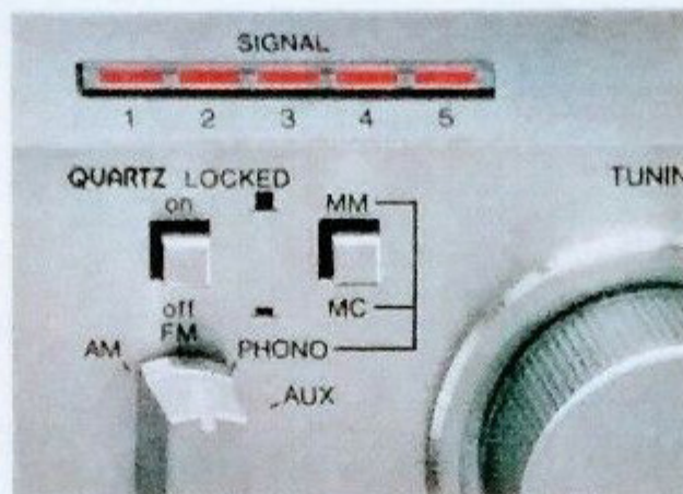
LED signal strength meter. Quartz locked tuning. Moving coil phono cartridge capability.
