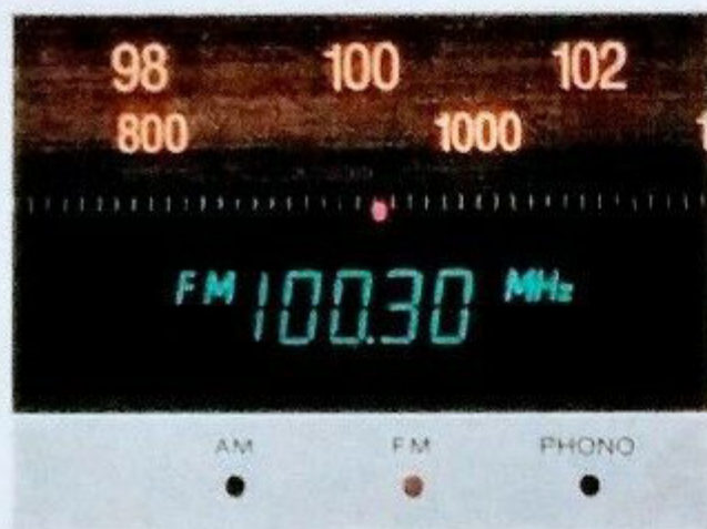
Sanyo's exclusive fluorescent Digital Plus display moves with dial pointer.
