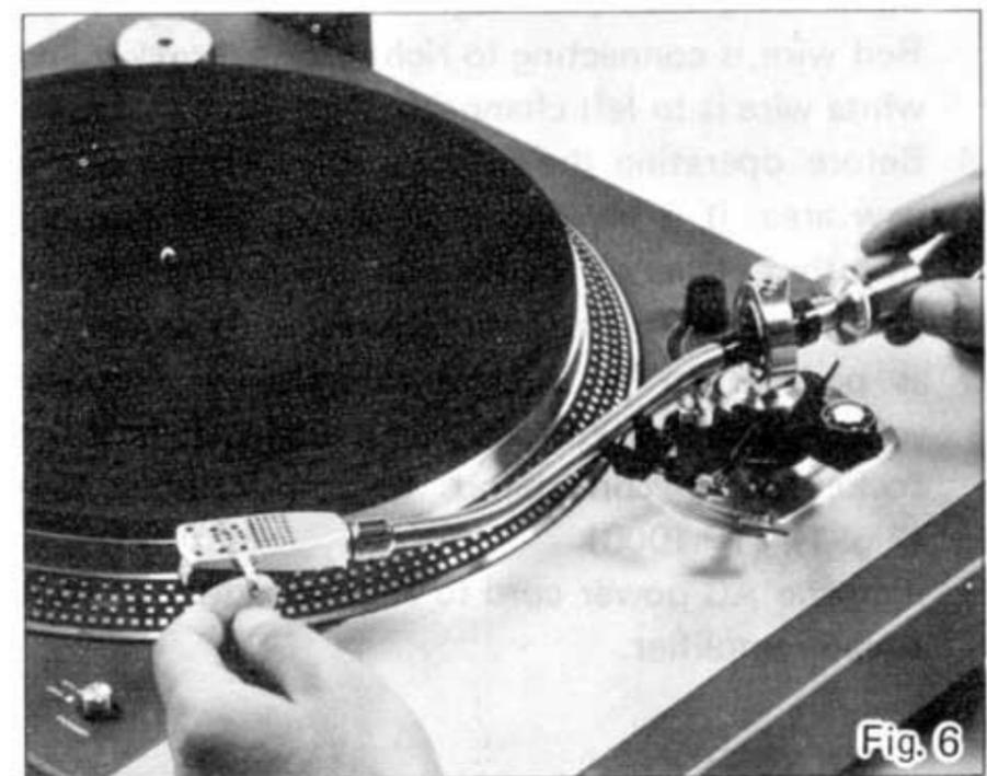
2. If it is hard to balance the tonearm horizontally only in use of main weight, use the sub-weight.
