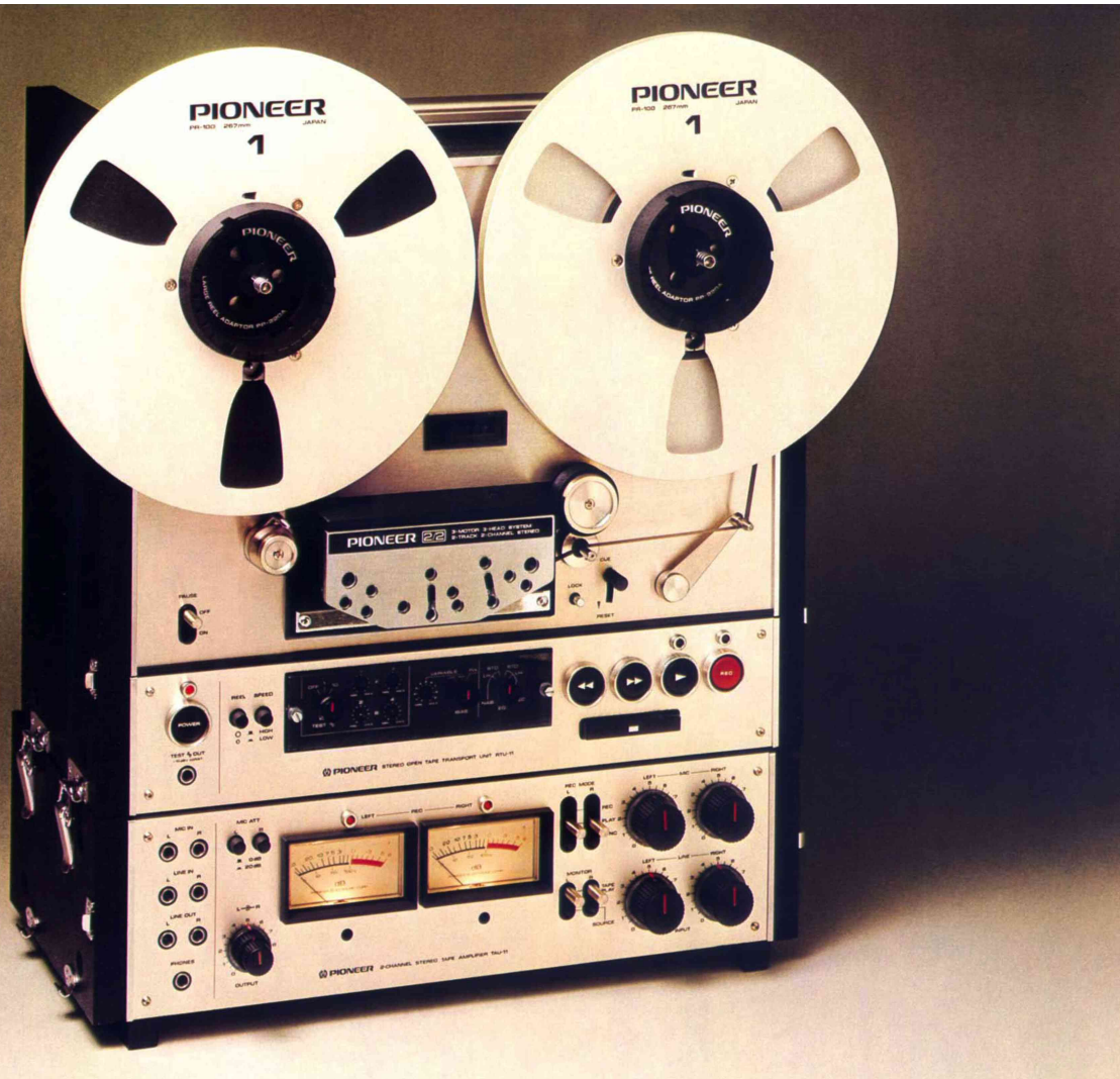
RT-2022: Professional open reel tape system. 2 tracks, 2 channels, 3 motors. Capstan drive. 38 cm/sec. and 19 cm/sec. Wow and flutter: no more than 0.04 % (JIS). Signal to noise ratio : more than 57 dB. Frequency réponse : 30 Hz to 28 kHz ( \pm 3 dB at 38 cm/sec.). Separate read unit. Separate record and playback amplifier.
