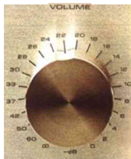
Main volume control with 22 contact points calibrated in decibels
