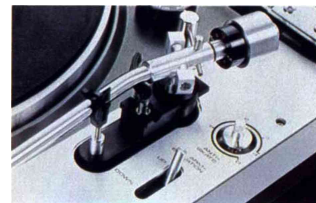
Tonearm pivot with anti-skating control.
