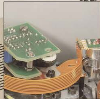
RaPos (Radial Positioner) - the professional way to achieve very fast access times.
