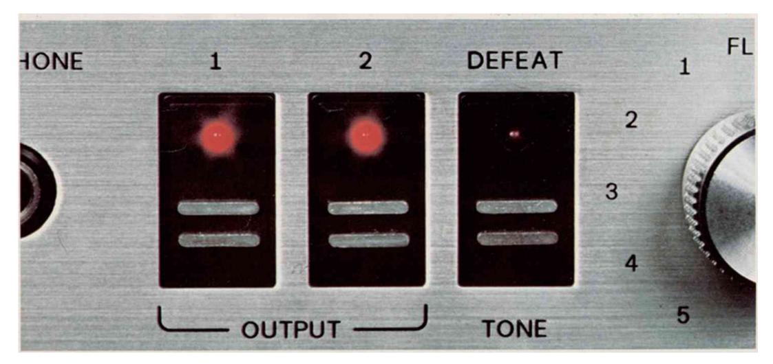
trols in a Baxandal feedback circuit allow the user to vary the frequency response in 2dB steps with the mid-position perfectly flat. A touch operated tone defeat switch duplicates the flat response of the mid-control position. Sophisticated electronic switching allows the tone defeat to fade in and out eliminating annoying clicks and pops.
