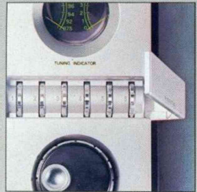
Setting wheels for station storage. Stored stations can be called up at any time using electronic Tsp buttons.
