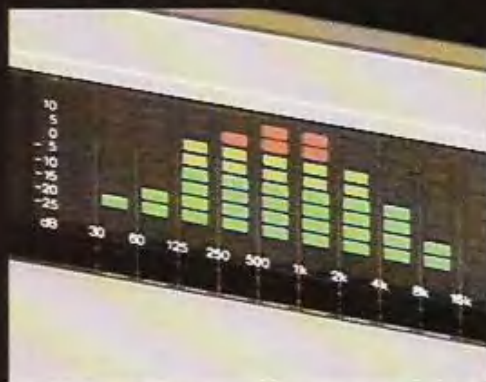
The audio spectrum analyzer in the SX-9100H/HB
