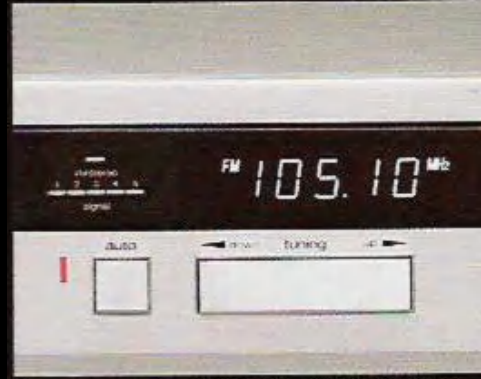
Quartz synthesizer tuner display provides clear indication of FM, MW and LW stations.
