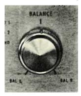
Right . . . turning the control to the right accents the right channel by reducing the left channel output.
