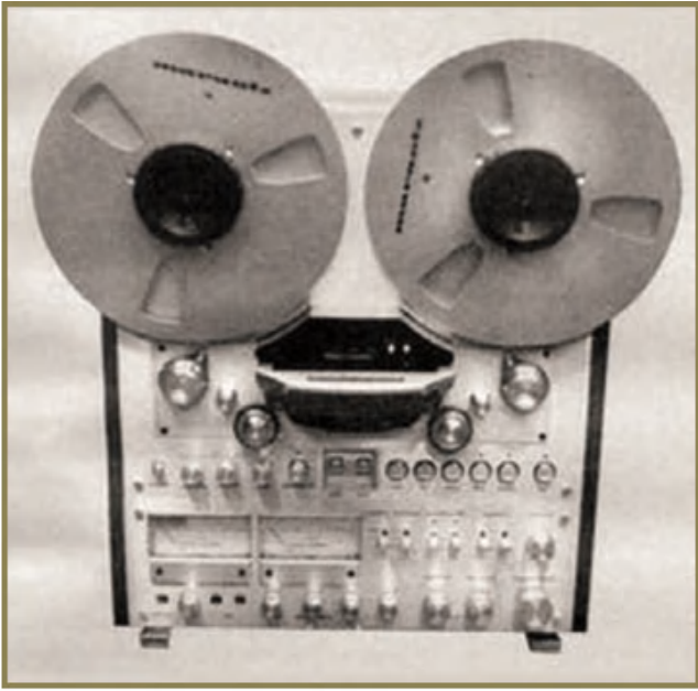
Marantz Model 7700 Tape Deck (1978), a three speed auto reverse unit. (Photo courtesy of http://www.classic-audio.com )
