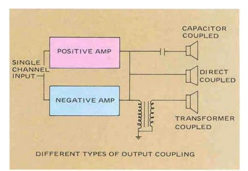
The direct coupled power output circuitry used in Marantz receivers has eliminated the need for coupling transformers and capacitors and the sound inaccuracies they can cause!'
