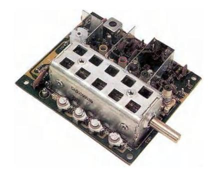
Superior selectivity is assured by a five-gang tuning capacitor in the Marantz 2325 and 2275 and a four-gang in the 2250B. A triple-tuned RF interstage on Models 2325 and 2275 and a dual-tuned RF interstage on Model 2250B provide excellent image and spurious response rejection.
