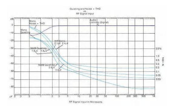
Two tuners with comparable weak signal sensitivities, but significantly different quieting slopes. Tuner A, with an IHF sensitivity of 2.4 uV. appears to deliver slightly less performance than tuner B. with an IHF sensitivity of 2.1 uV, or specified 0.3 uV better. However, tuner As steeper quieting slope indicates that it gets quieter, fasferthan tuner B— a significant advantage under actual performance conditions.
