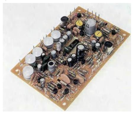
A phase locked loop FM multiplex demodulator is used in all Marantz receivers for low distortion, excellent stereo separation and superior noise rejection:
