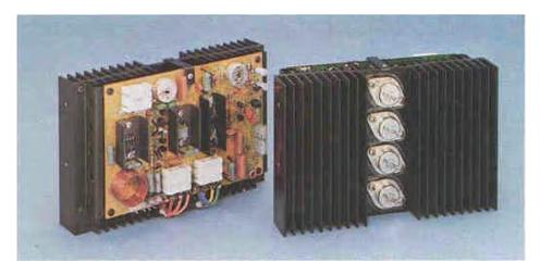
Full complementary symmetry output assures higher stability, better linearity and lower distortion than the quasi-complementary outputs in most receivers!
