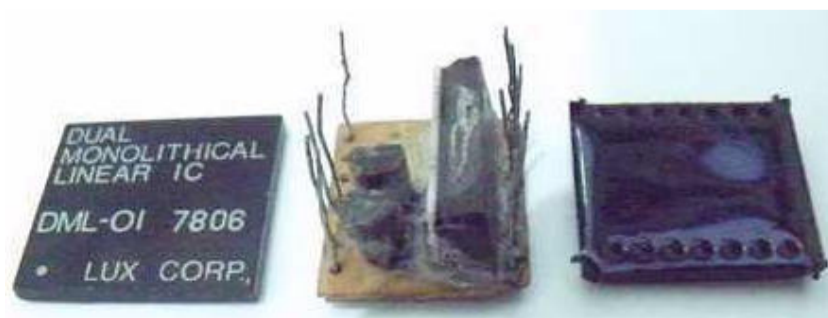
The whole assembly of the DML, the resin removed ^
