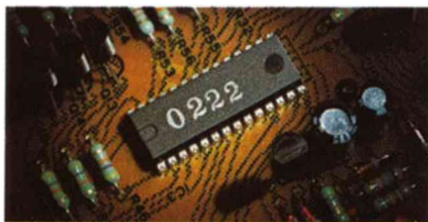
The "brain" that controls tonearm action.
