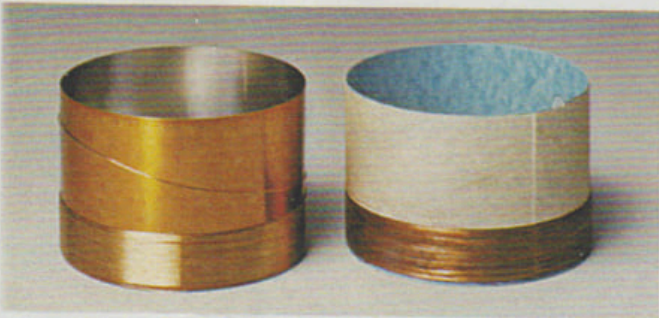
LEFT: Kenwood Aluminum Voice Coil Bobbin RIGHT: Conventional Kraft Paper Bobbin Aluminum voice coil bobbin provides high thermal conductivity for better heat dissipation, lets the speaker handle higher input loads.
