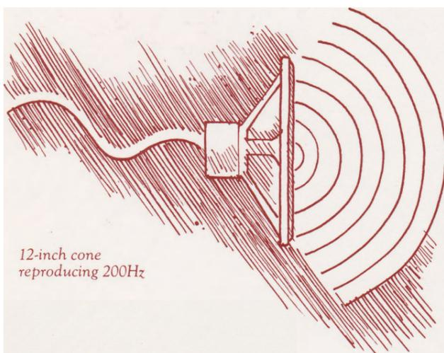
At a frequency of 2000 Hz, the wavelength is only about 7 inches. If the same 12-inch cone were made to reproduce that frequency, it would be focused into a beam.
