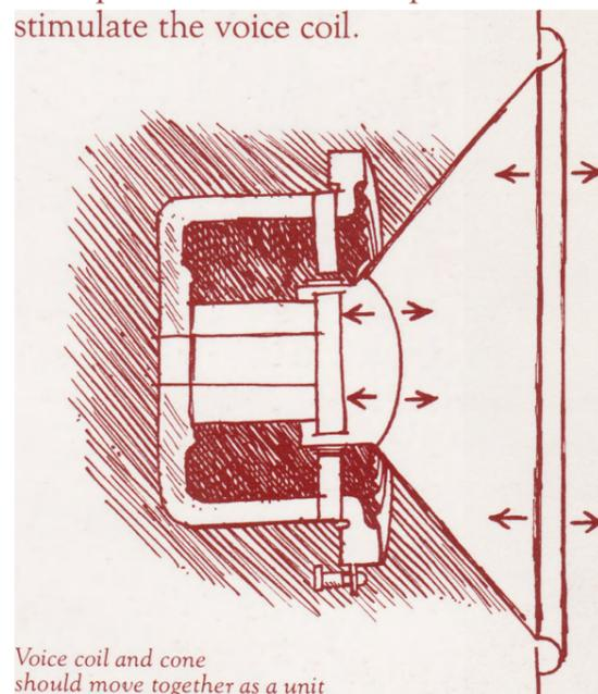
Voice coil and cone should move together as a unit
