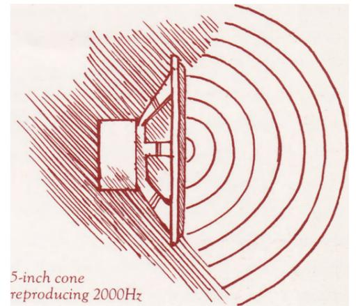
The dispersion limitation on the 5-inch midrange does not become acute until the frequency has reached around 8000 Hz. So, typically above 6500 to 7000 Hz, frequencies are directed by another cross-over network to a tweeter with a diameter of approximately  $1\frac{1}{2}$  inches. Again, wide dispersion. But only up to a point. When wavelengths approach  $1\frac{1}{2}$  inches, the usual tweeter will be unable to disperse them. Radiation starts to focus into a narrow beam.
