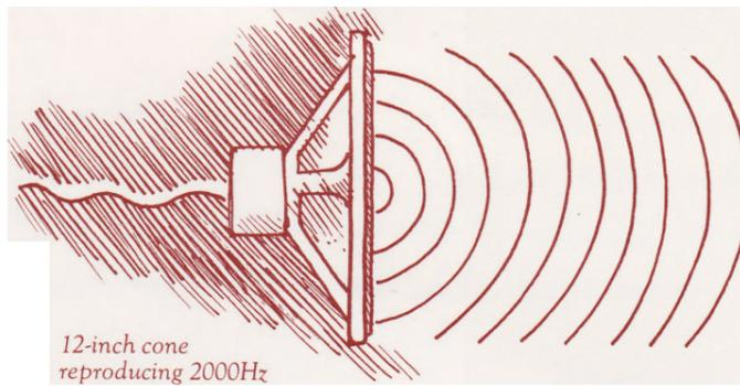
The listener would be able to hear 40 Hz reproduced by that 12-inch cone from any position in the room. He could hear 200 Hz over a wide area of the room, but to properly hear 2000 Hz, he should be nearly on axis, or in a straight line from that loudspeaker.
