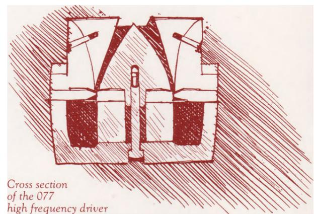
The 077 has unusually high efficiency as a result of hornloading, but the significance of the horn is much greater when its effect on dispersion is considered. In professional use, this assembly has been variously called a slot radiator and a diffraction horn. In fact, the horn is a very unusual development combining a tried and true idea: basically it's an exponential horn, but it incorporates diffraction characteristics.
