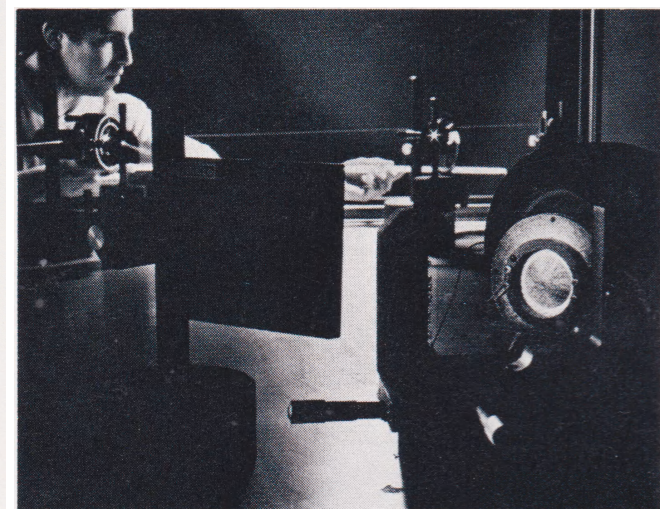
In the JBL laser laboratory, holograms are used to study the behavior of loudspeaker components under operating conditions.
