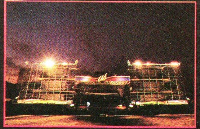
More than 2,400 individual loudspeaker components made up the 400,000 Watt JBL sound system built to power the three-day "US Festival" in Southern California. Critics from music industry publications called the system "the best outdoor sound system ever constructed."
