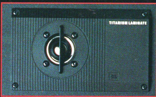
Borrowing from the acclaimed "Ti" Series, all JBL home loudspeaker systems use titanium—a material that is harder than steel, yet half the weight—in the construction of the high frequency transducers.
