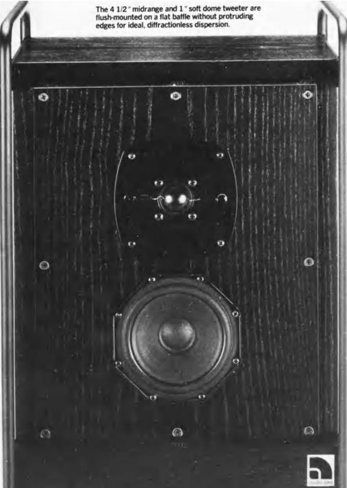
power amplifiers. One is used for the built-in ACE-Bass subwoofer, which handles frequencies from 30 Hz (-3 dB) to 300 Hz and the other feeds the midrange driver and tweeter.
